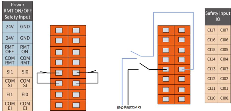
Figure 6-8 Safeguard Stop Reset Input Connection
