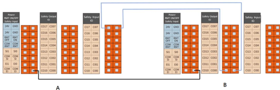
Figure 6-13 System Stop Input Connections (from B to A)
