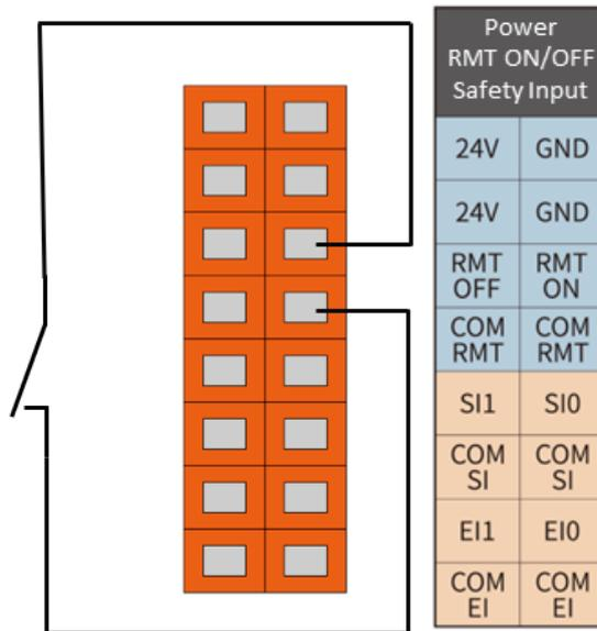
Figure 6-30 Remote power-on connection
