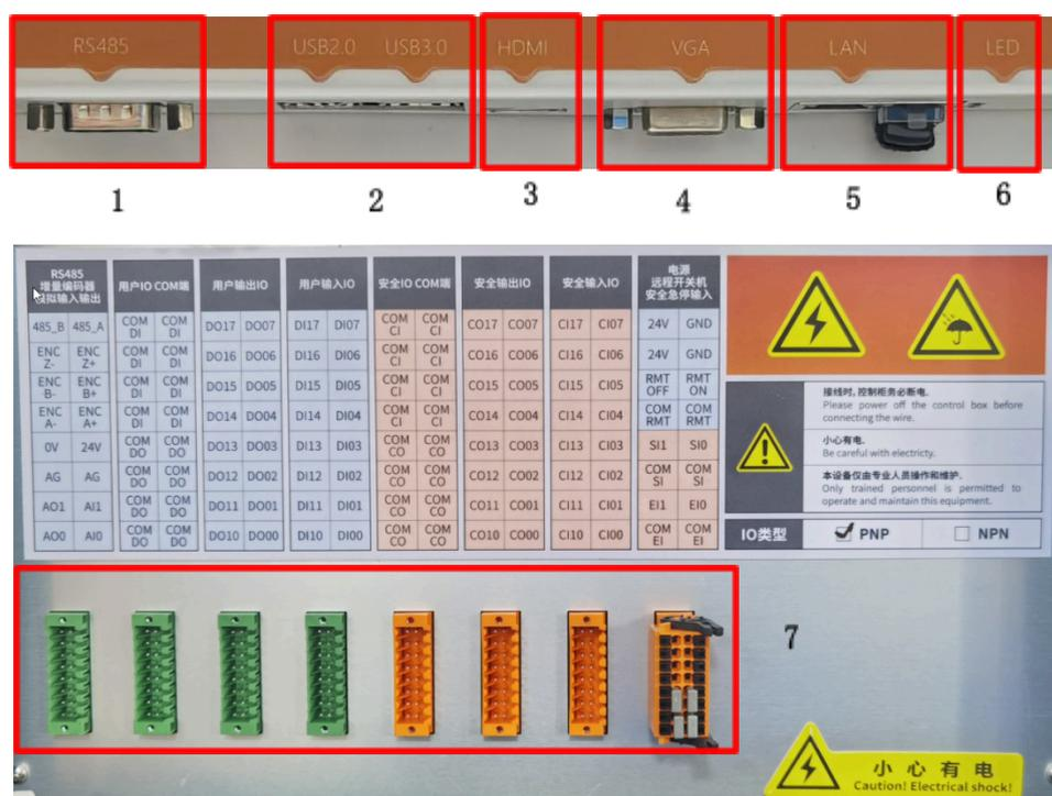
Figure 6-1 Control Box Internal Interfaces
