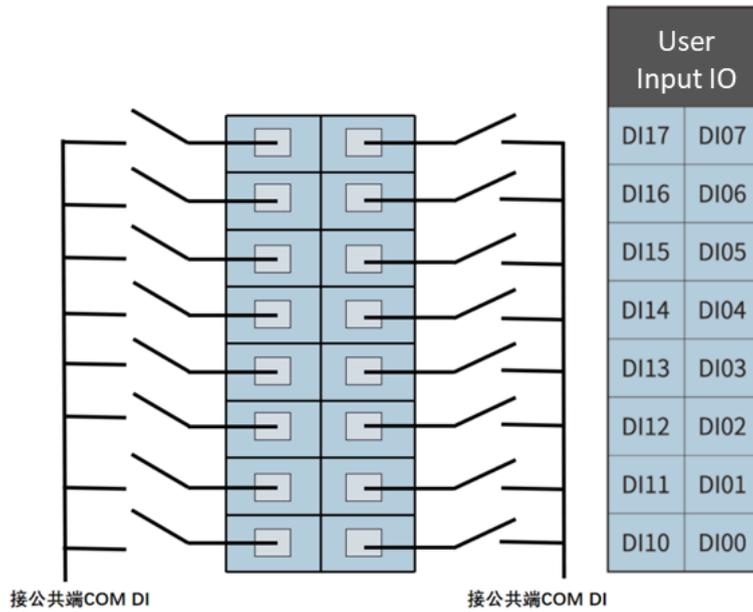
Figure 6-23 DI terminal connection button switch
