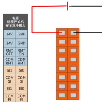
Figure 6-4 Schematic diagram of external power supply
