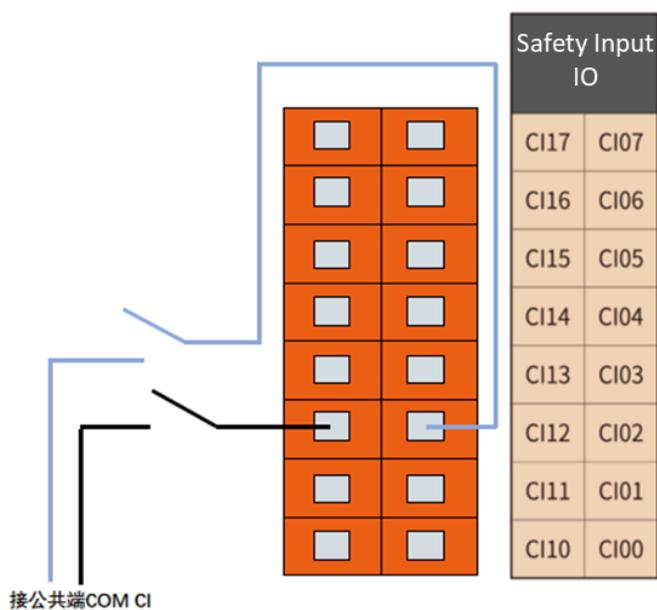
Figure 6-7 Reduced mode input
