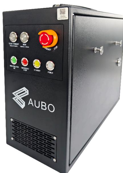
Figure 5-1 AUBO-iS control box appearance
