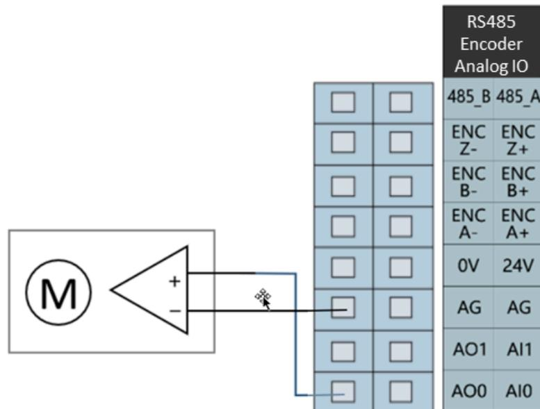
Figure 6-28 Analog voltage output connect drive device
