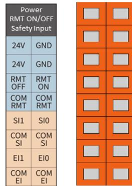
Figure 6-29 Remote control I/O interface
