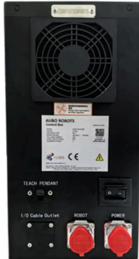
Figure 5-3 Rear panel of the control box
