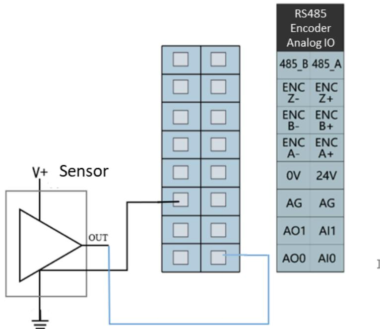
Figure 6-26 Analog I/O interface diagram
