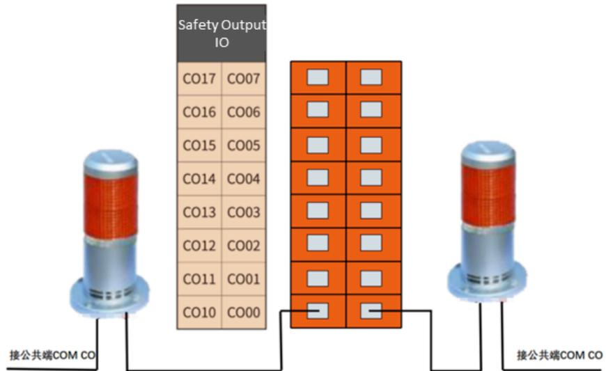
Figure 6-14 System emergency stop output
