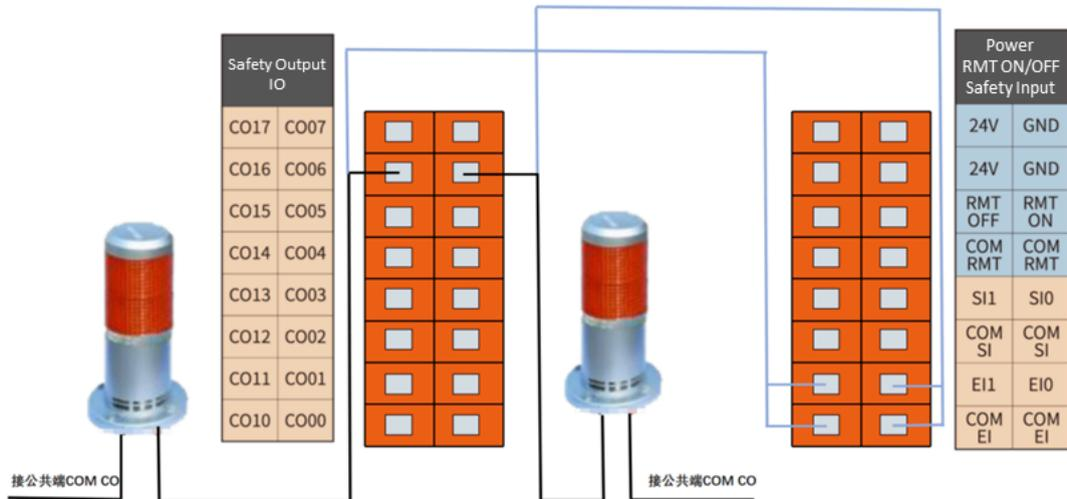
Figure 6-20 Multiple robots sharing emergency stop
