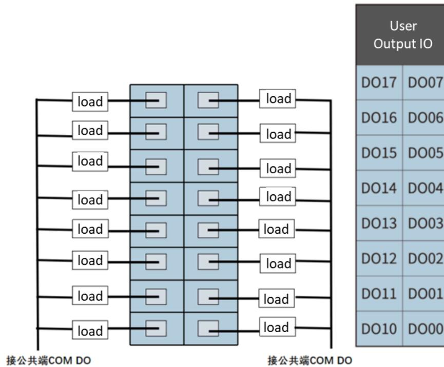
Figure 6-25 DO Terminal Load Interfacing Schematic Diagram
