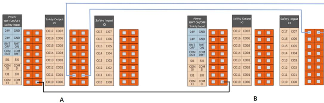
Figure 6-12 System Stop Input Connections (from A to B)
