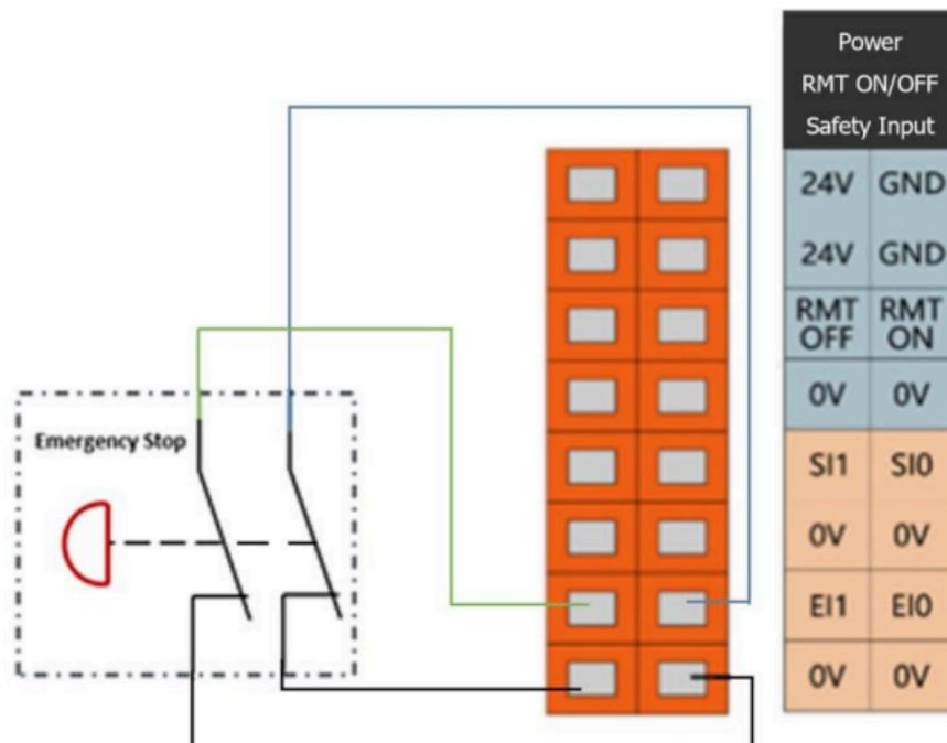
Figure 6-5 External emergency stop input
