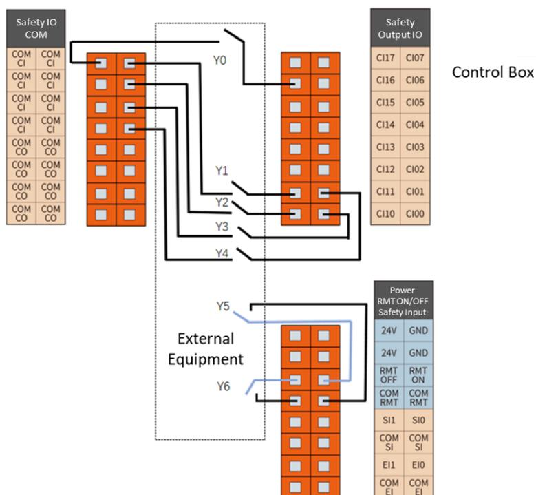
Figure 6-32 Linkage control I/O connection
