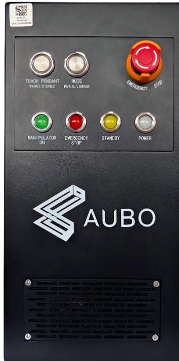
Figure 5-2 Control box front panel
