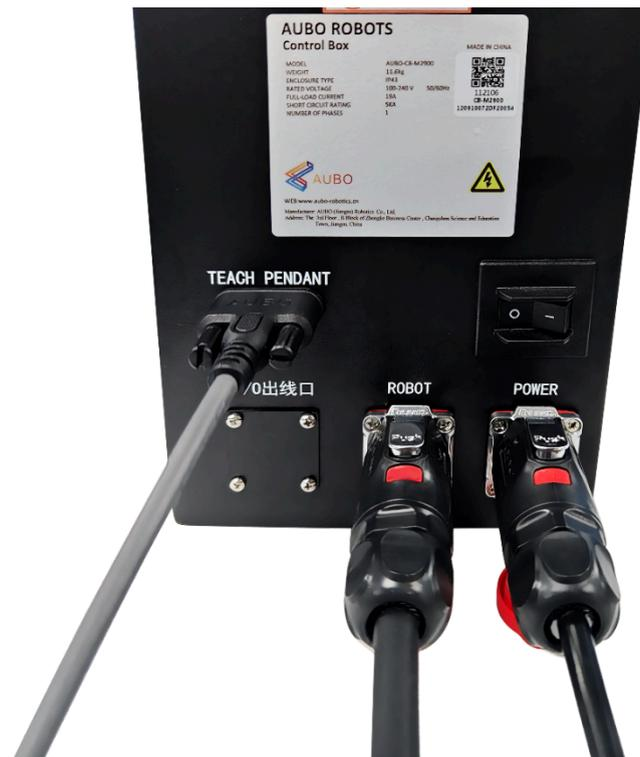
Figure 5-4 Cable connection of the control box
