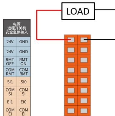
Figure 6-3 Schematic diagram of internal power supply
