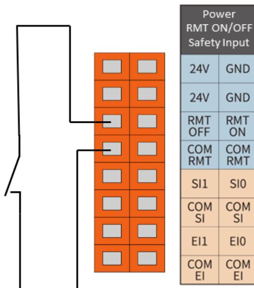
Figure 6-31 Remote shutdown connection
