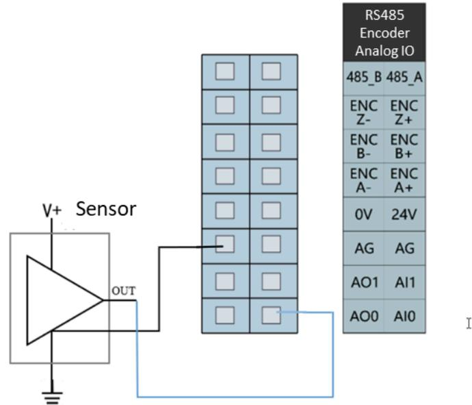
Figure 6-27 Analog voltage input connected to a sensor
