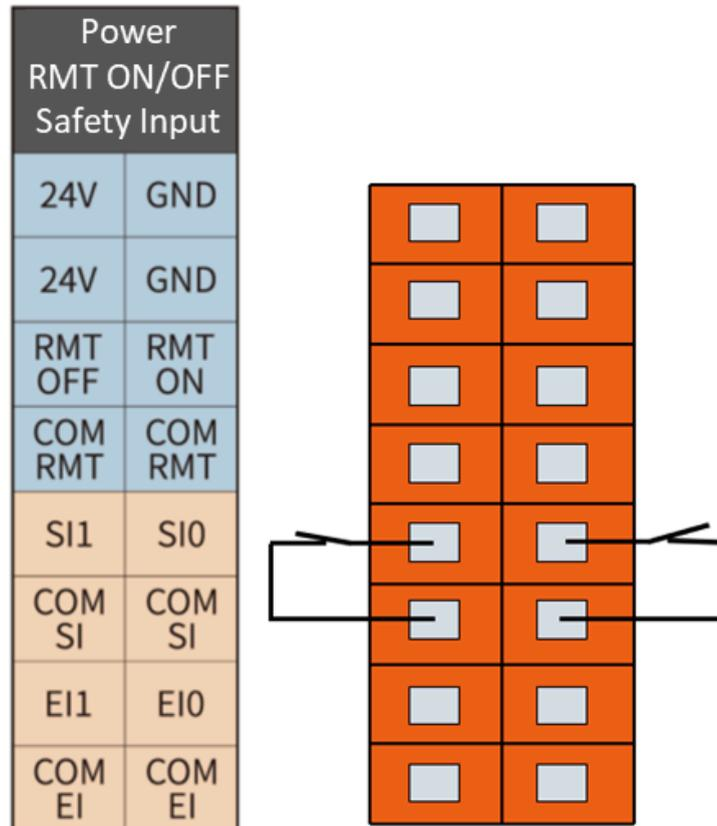
Figure 6-6 Diagram of protection stop input connection
