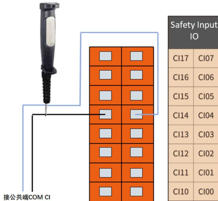
Figure 6-9 Enabling device input
