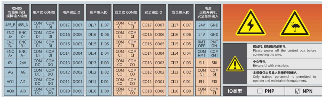
Figure 6-2 I/O Factory Preset Logic-Level Configuration Diagram
